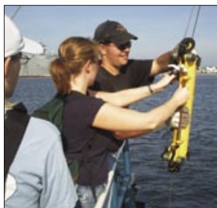
"The salinity is on the right, in parts per 1,000," yells Roger Harrington over the engine noise. He takes turns with lab-cruise instructor Johnny Waugh, teaching use of a hand refractometer to measure water chemistry and to operate the soil sampler that drags the sea bottom.
